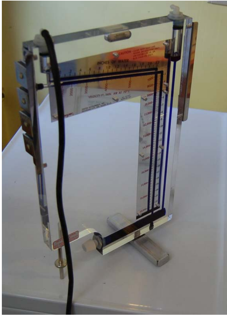
Figure 3: Test setup - Inclinometer
