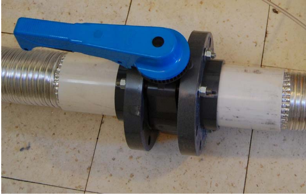
Figure 4: Photo showing standard metal flexible dryer venting hose and restricting valve in line to simulate lint buildup.
